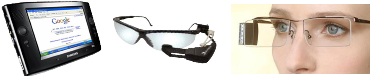
Figure 3. Examples of augmented reality display devices: hand held units and see through HMD.
