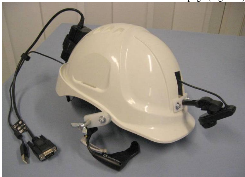
Figure 7. The modified helmet with Micro Optical SV-6 HMD and Logitech web camera.
