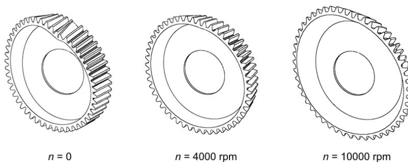
**Figure 4. Thin-rimmed gear displacement (scaled) at 0, 4000 and 10000 rpm**
