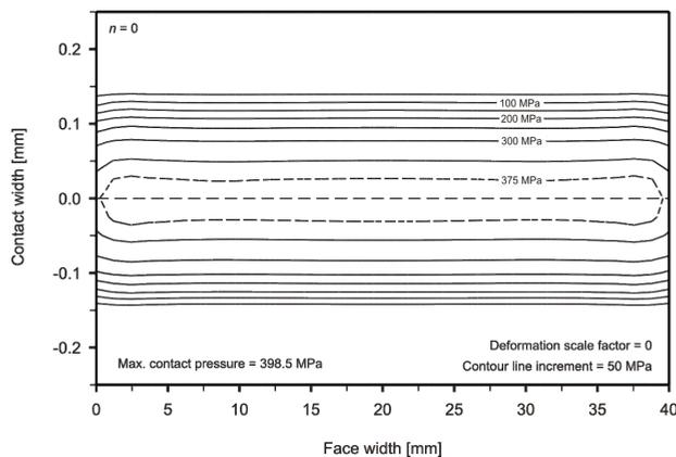
**Figure 1. Contact pressure contour lines for solid spur gears engaged**
