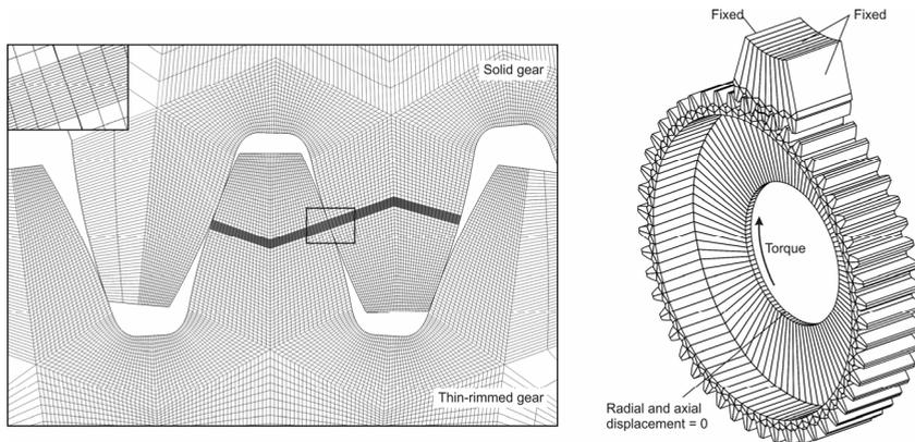
Figure 3. Model used in FEM analysis along with refined mesh detail
