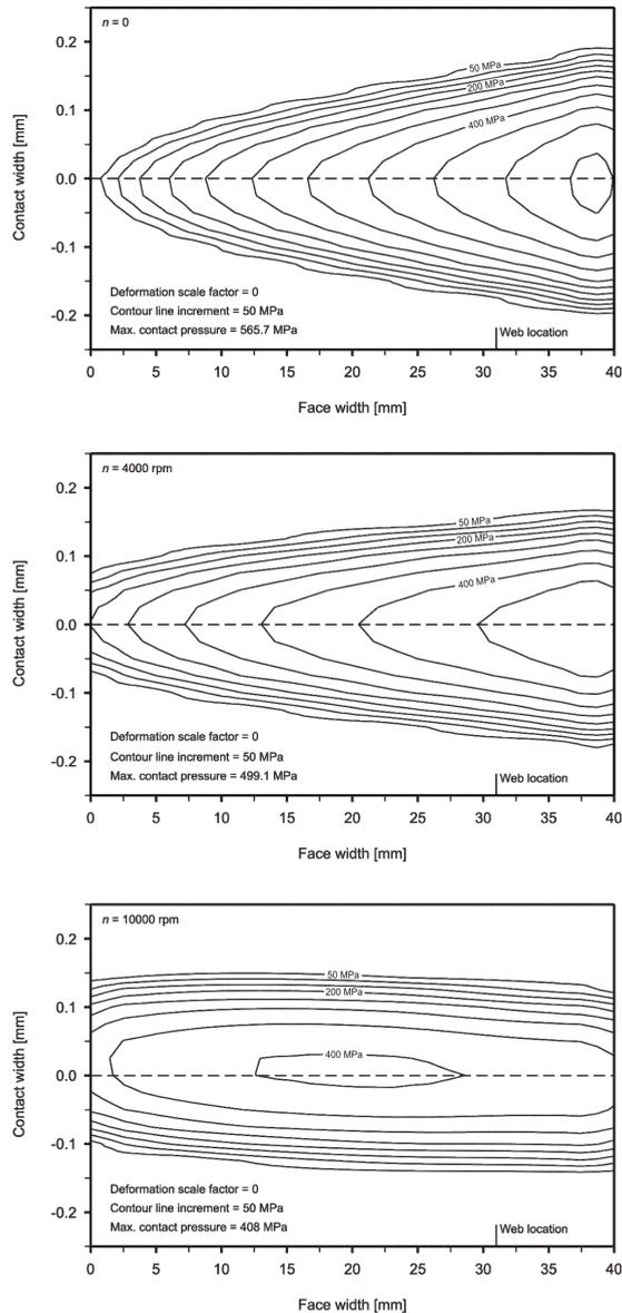
**Figure 5. Contact pressure contour lines for thin-rimmed gear at 0, 4000 and 10000 rpm**
