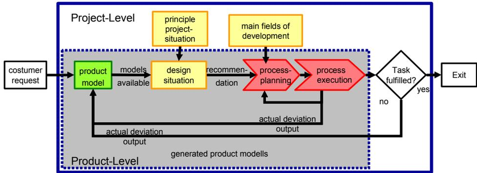
Figure 1. Generic process model for specifying the decision making (according to [2])
