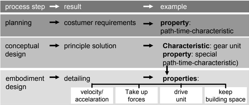
**Figure 3. Coupling of previous stages in the product's development with characteristics**
