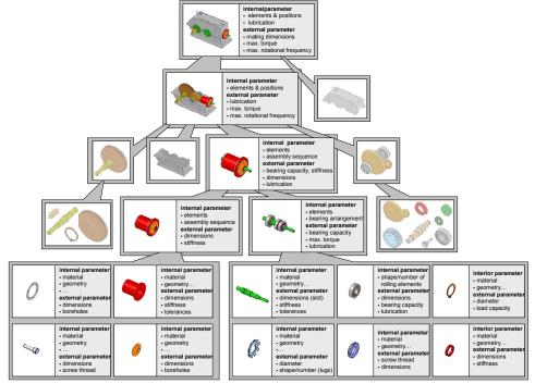
Figure 2. Structure of a transmission
