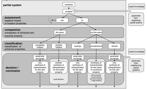
Figure 3. Microcycle based on property-driven parameter exchange
