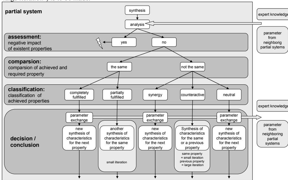
**Figure 3. Microcycle based on property-driven parameter exchange**
