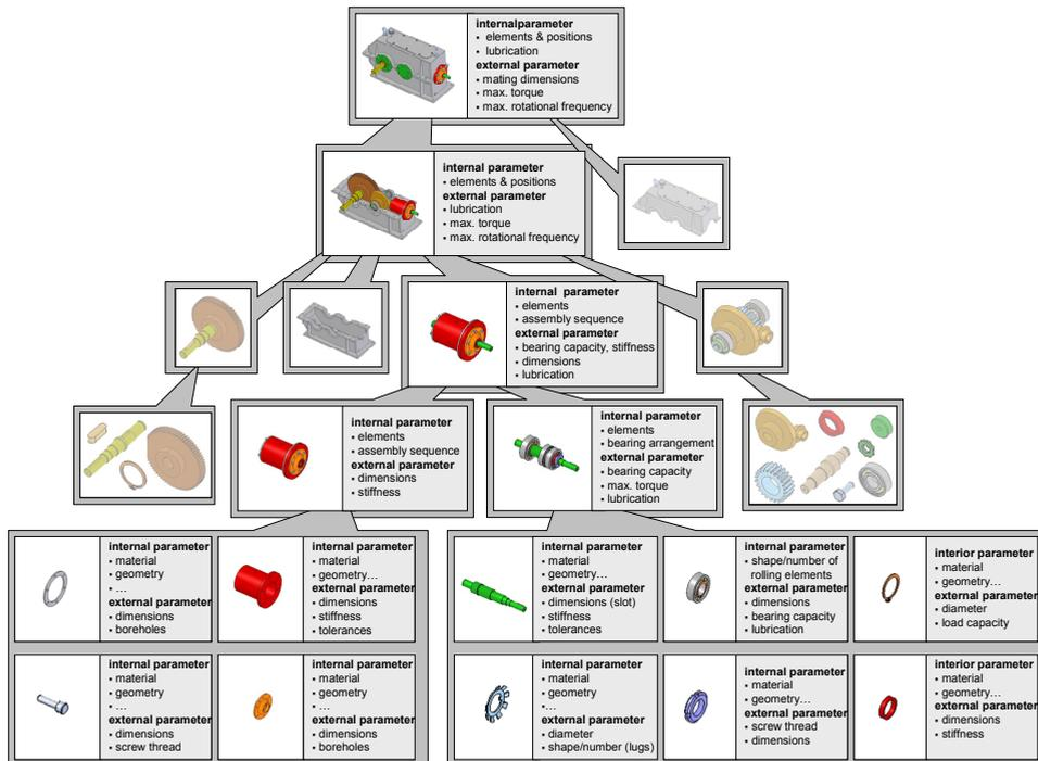
Figure 2. Structure of a transmission
