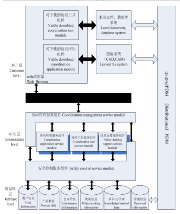
图1 基于Web的协同工作平台体系结构 Fig.1 The architecture of Web-based collaborative
