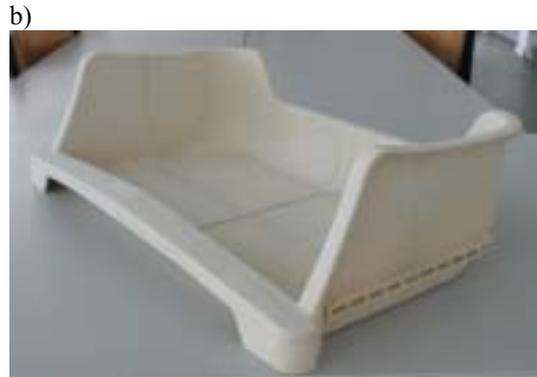
Fig. 2. Models produced with use of 3DP technique (divided on small parts and glued together): a) front panel from fridge (width 600mm), b) drawer from freezer (width 480mm).
