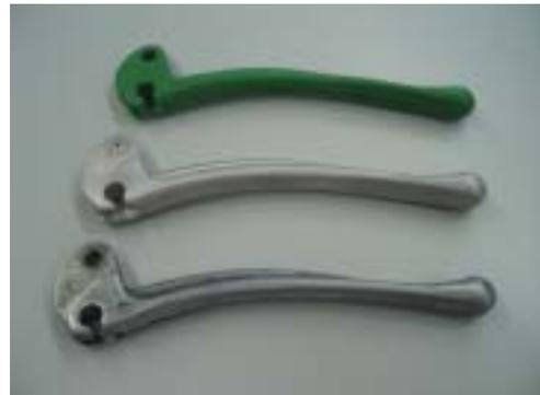
Fig. 4. Prototypes produced with use Vacuum Casting technique: a) silicone mould with wax model; b) brake lever: from resin, from low melting alloy, original – aluminum.
