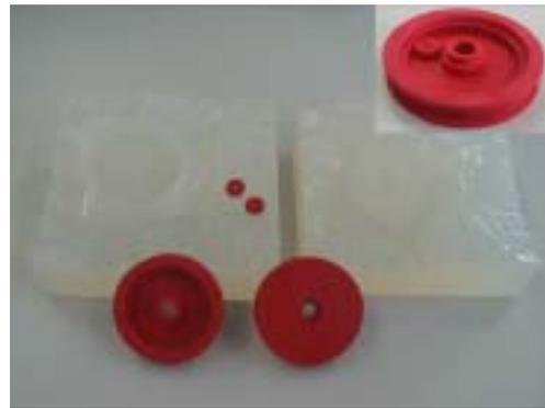
Fig. 5. Prototypes produced with use Vacuum Casting technique: a) resin jar original - produced in 3DP technique (black) and resin prototypes casted in silicone mould; b) silicone mould and resin cogs (wheels).
