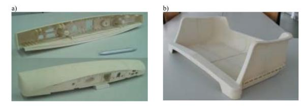
Fig. 2. Models produced with use of 3DP technique (divided on small parts and glued together): a) front panel from fridge (width 600mm), b) drawer from freezer (width 480mm).
