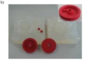
Fig. 5. Prototypes produced with use Vacuum Casting technique: a) resin jar original - produced in 3DP technique (black) and resin prototypes casted in silicone mould; b) silicone mould and resin cogs (wheels).
