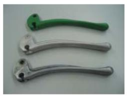
Fig. 4. Prototypes produced with use Vacuum Casting technique: a) silicone mould with wax model; b) brake lever: from resin, from low melting alloy, original – aluminum.
