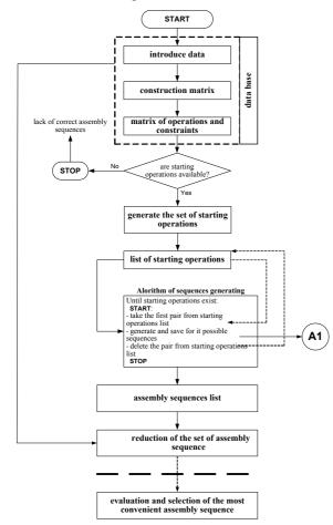
Fig.5. Algorithm of assembly sequence assignment
