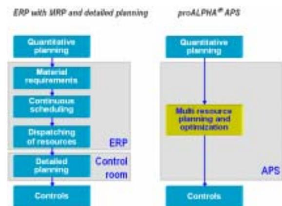
Fig.1. Comparison of MRP and proALPHA<sup>®</sup> APS
