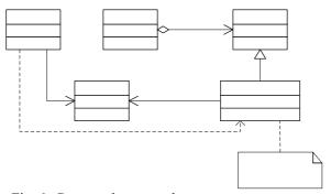
Fig. 6. Command pattern class structure
