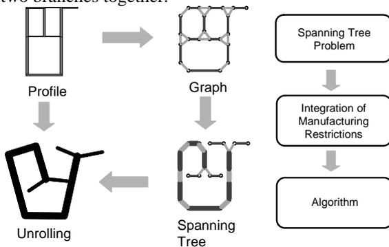
Figure 6. *Modelling the cross-section as a spanning tree-graph*
