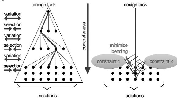
Figure 2. Human and algorithm-based design approach for the early phases of design
