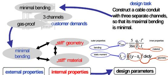
Figure 3. Transforming a verbal design task into an equation as a formal description
