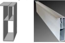
Figure 8. The 3D-CAD model of the cable conduit (left) and the final product (right)
