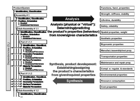
Fig. 1. Characteristics (left) and properties (right) with analysis and synthesis as the two main relations between the two
