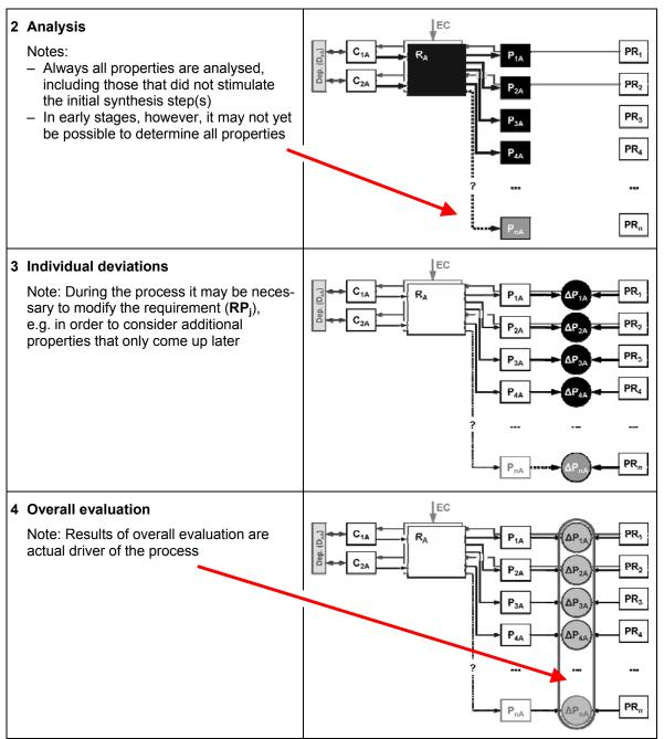
Fig. 6. PDD-scheme of steps in the first cycle ("cycle A") of product development
