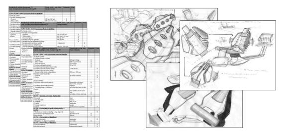
Figure 4. Integrated List of Requirements with textual and graphical parts - Example: Dental Chair
