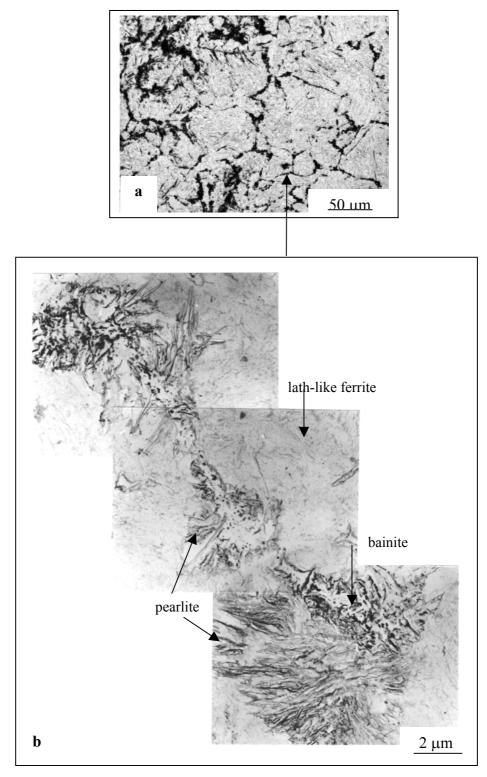
Figure 4. Steel 0.5C-1Cr-0.8Mn-0.3Si, the heavy strained central part of specimen deformed at 650°C and hold at isothermal dwell at 350°C for 70s. a) OM micrograph of metallographic sample, b) TEM micrograph of carbon extraction replica.
