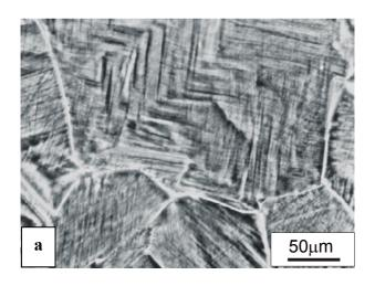
Figure 1. Steel 18Cr18Mn0.5N deformed by tension at a total strain of 0.15 at room temperature.
