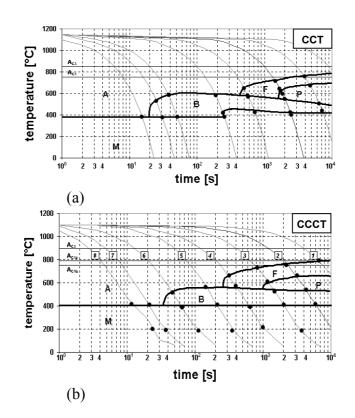
Figure 2. Transformation diagrams of steel 0.2C-0.7Cr-0.9Mn-0.4Mo: a) continuous cooling transformation diagram (CCT), b) continuous cooling compression transformation diagram (CCCT).
