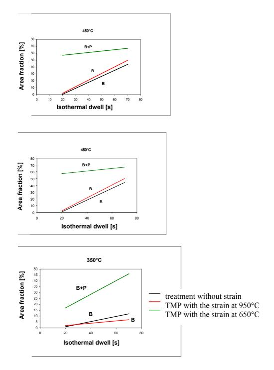
Figure 3. Resultes of quantitative microstructural evaluation of steel 0.5C-1Cr-0.8Mn-0.3Si. Area fraction of bainite (B) and pearlite (P) after different methods of heat treatment or thermo-mechanical processing with isothermal dwell at 450°C, 400°C a 350°C.
