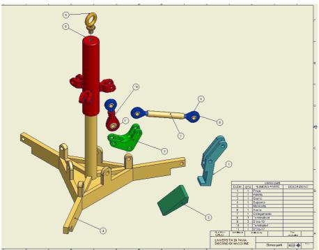
Fig. 3. Parts and assembly realised by students.
