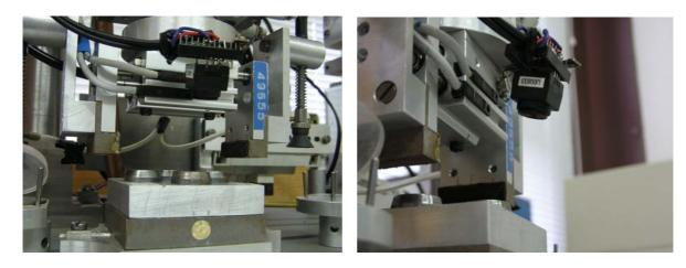
Figure 11. Camera module on the handling arm
