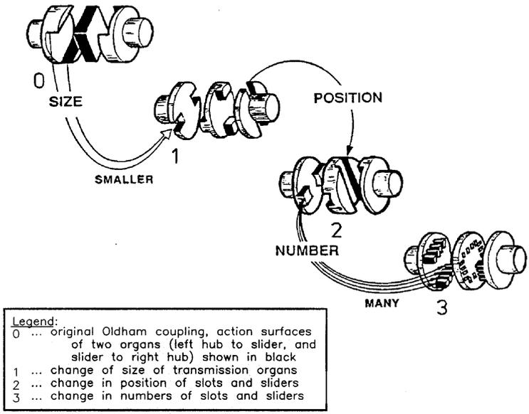
NOTE: Oldham couplings provide a rotational connection between two shafts and allow small angular mis-alignment.
