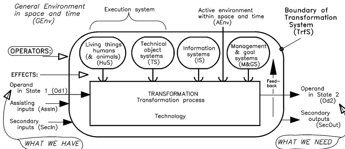
**Figure 1. General Model of a Transformation System**
