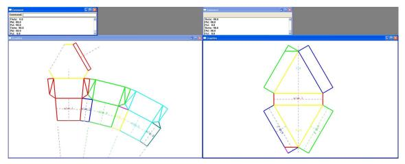
Figure 6. Generic carton simulation showing carton net for six sided gable top skillet (left) and triangular carton (right)
