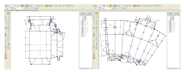
Figure 4. Constrained parametric nets created within a commercial CAD system showing corner gussets (left) and gable top (right)
