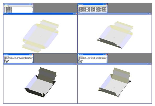
Figure 7. Origami tray shown flat (top left), with folds resulting from a single ground line rotation (top right), four simultaneous ground folds with gussets forced inwards (bottom left) and outwards (bottom right).
