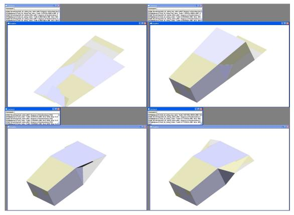
Figure 8. Showing a gable topped skillet carton showing similar erection processes
