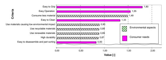
Figure 8: Criteria priority for 'housing-upper side' of computer mouse
