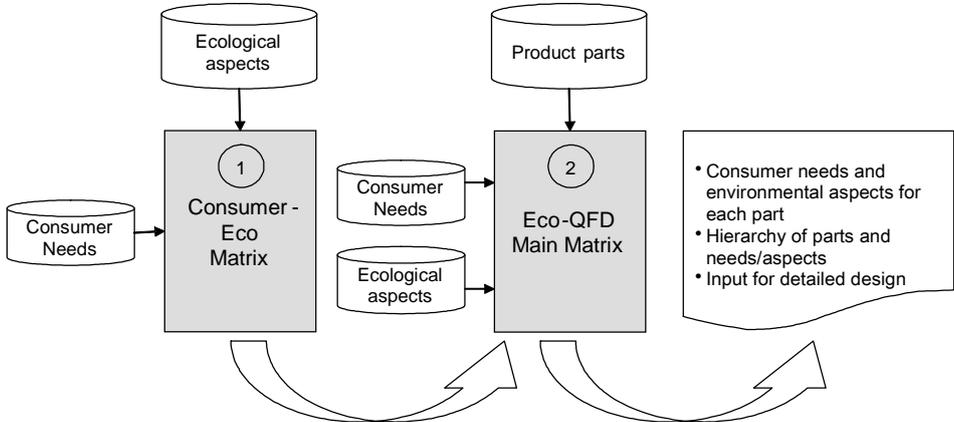
Figure 3: Structure of the Simplified Eco-QFD
