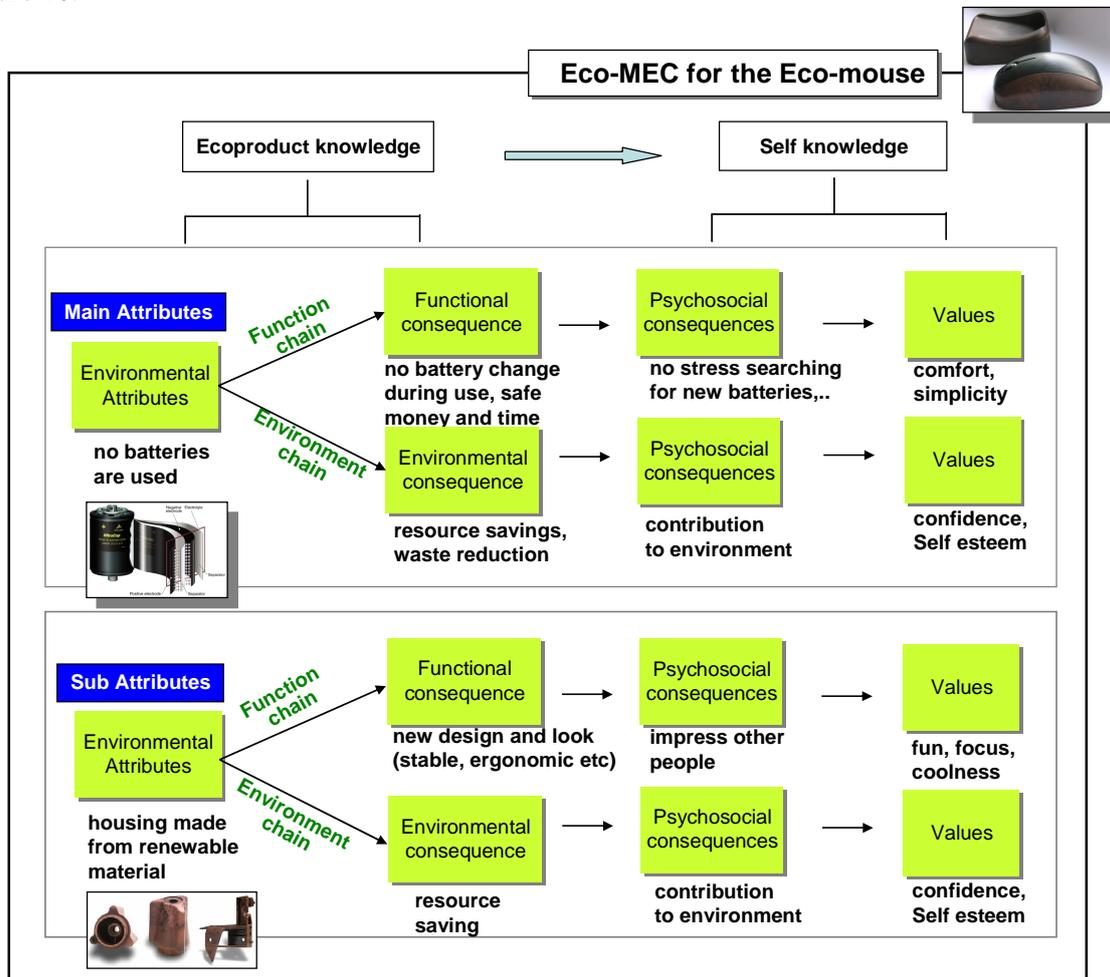
Figure 10: Eco-MEC for the eco-mouse (ref. the Eco-MEC Model [18])
