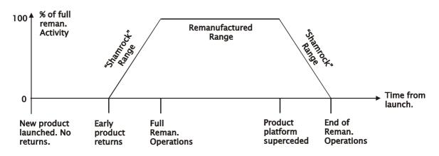
Figure 5: The Xerox Remanufacturing Ramp Up/Down for each Product Line
