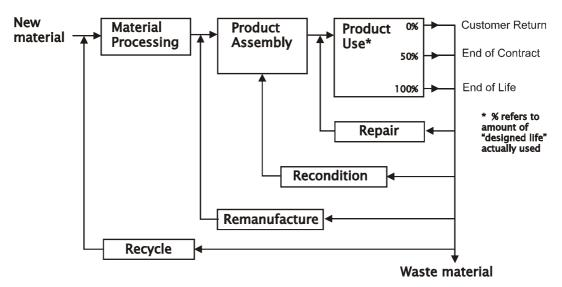
Figure 1: Closed loop design through repair, remanufacturing or recycling
