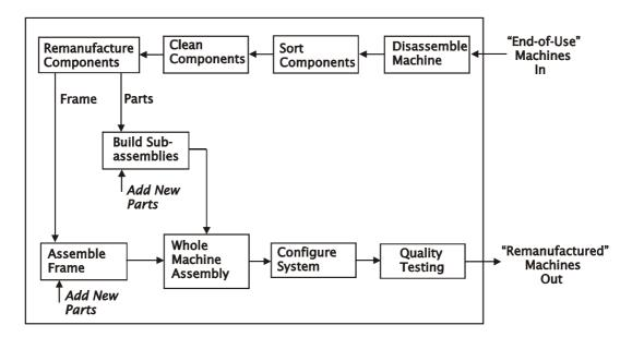
Figure 3: Xerox Dundalk's Remanufacturing Process Flow
