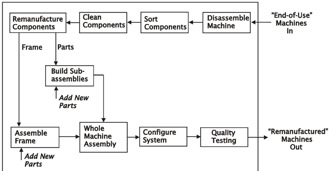
Figure 3: Xerox Dundalk's Remanufacturing Process Flow
