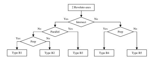
Figure 1. Binary tree displaying possible link topologies
