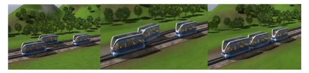
Figure 1. Railcab Shuttles forming a convoy
