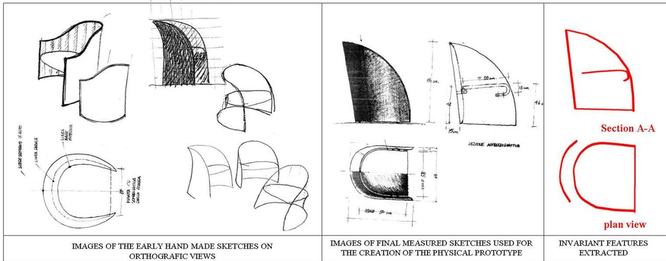
Figure 3: Searching for invariant curves (interpretative schemata) in the “Intervista” product. The early sketches are compared with the detailed ones in order to recognize the styling curves on the 3D dataset. The interpretative schemata are extracted in the same reference planes of the final sketches.
