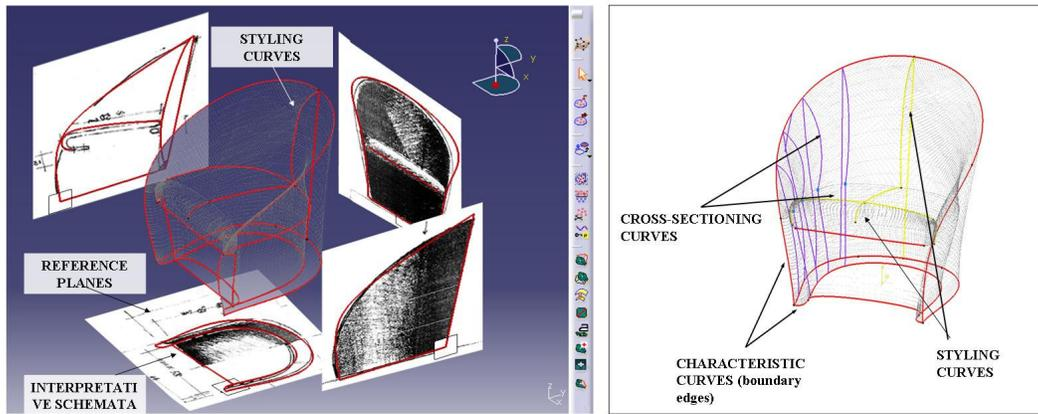
Figure 4: Extraction of the styling curves, characteristic and cross-sectioning curves from the 3D dataset
