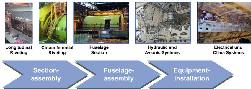
Figure 2. Main steps of the fuselage production process in Hamburg
