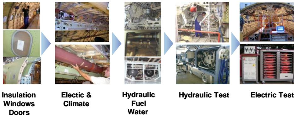
Figure 3. Equipment installation and test of fuselage systems
