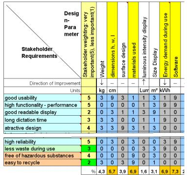
Figure 5. Step 4 - Quality Function Deployment [7]
