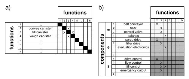
Figure 4. Simplified example of a weight controlled filling system:a) Illustration of the functional structure via DSM.b) Cross-linking between functions and components via DMM.
