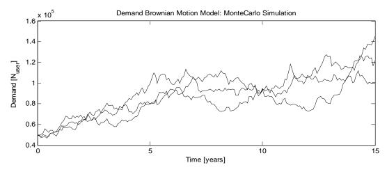
Figure 3: GBM model of uncertain demand,  $\Delta T$  = 1 month, D (t=0) = 50,000,  $\mu$  = 8% p.a.,  $\sigma$ = 40% p.a. – 3 scenarios are shown (from de Weck et al. 2004)[3]
