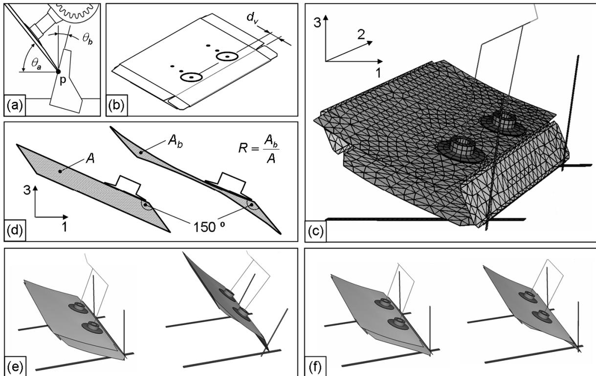
Figure 3. (a) Backstop orientation. (b) Vacuum cup locations (not to scale). (c) FE model of the carton and packaging machine. (d) Opening ratio calculation. (e) Typical appearance of the FE simulation with backstop at 0 (left) and 30 degrees. (f) Views of the FE simulation with vacuum cups positions closest (left) and furthest from the crease.
