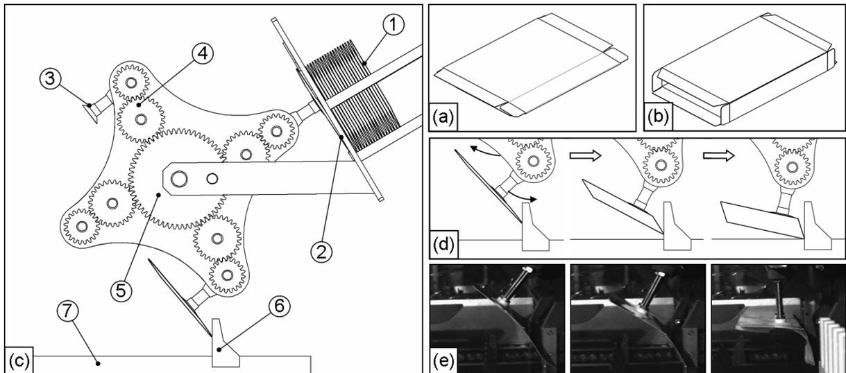
Figure 2. (a) Skillet. (b) Erected carton. (c) Erection mechanism showing skillets (1), feed aperture (2), vacuum cups (3), epicyclic gear train (4), sun gear (5), backstop (6) and fixed rails (7). (d) The mechanism erects the skillet by forcing one edge against the backstop. (e) Frames from high speed video footage of a carton failing in buckling.
