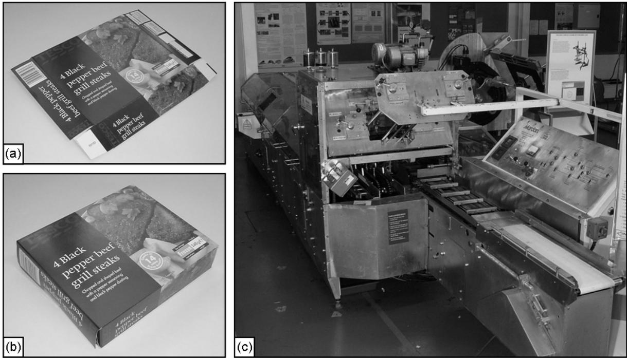
Figure 1. Skillets (a) are erected, filled and sealed to form shelf-ready cartons (b) by automated machinery (c) capable of processing over 250 packs per minute.
