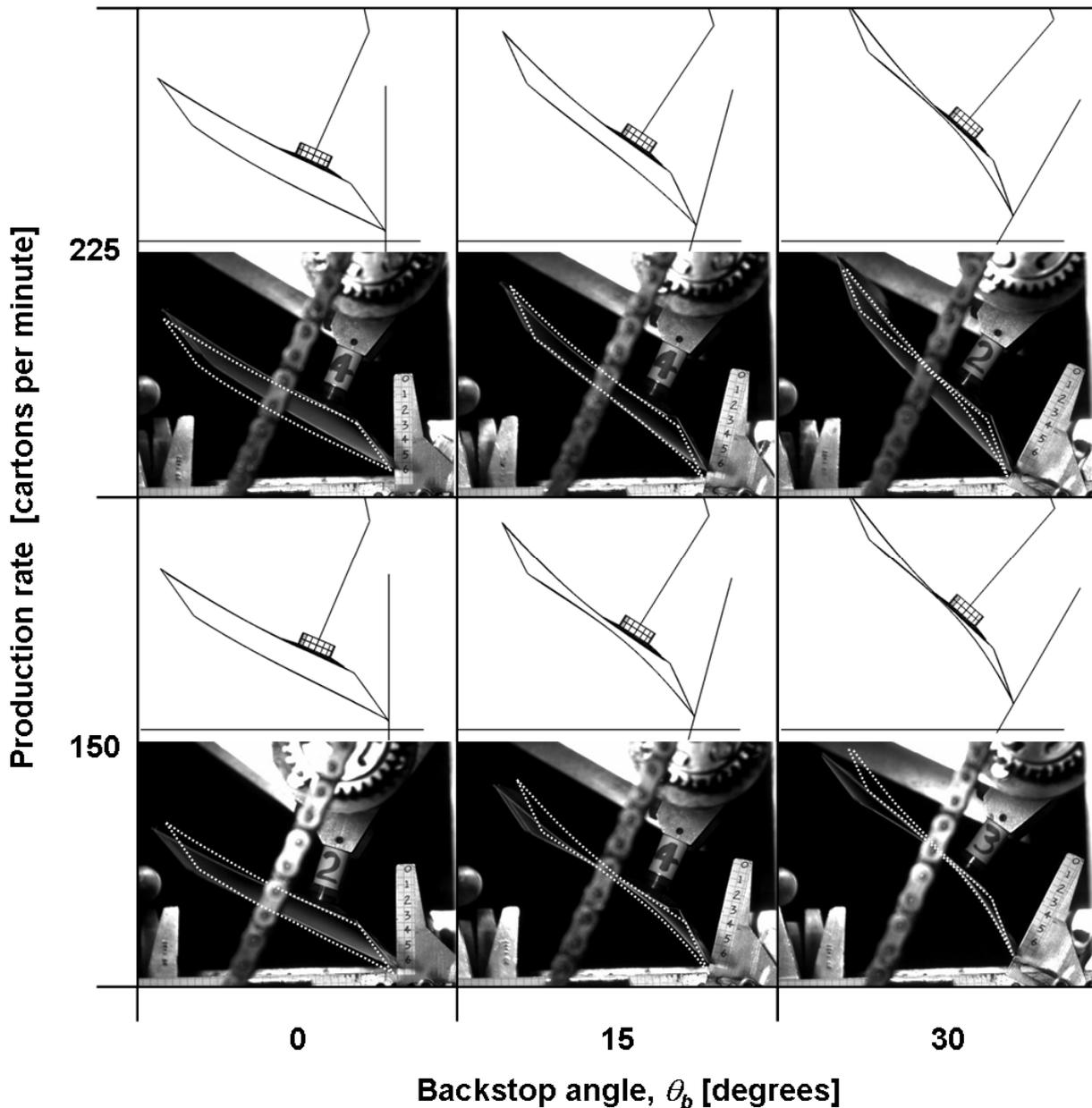
Figure 4. Comparing simulation results with high speed video footage of skillet erection at the three backstop angles considered. Predicted results are shown above corresponding frames from high speed video. Predicted results (dotted line) are superimposed on the high speed video images.
