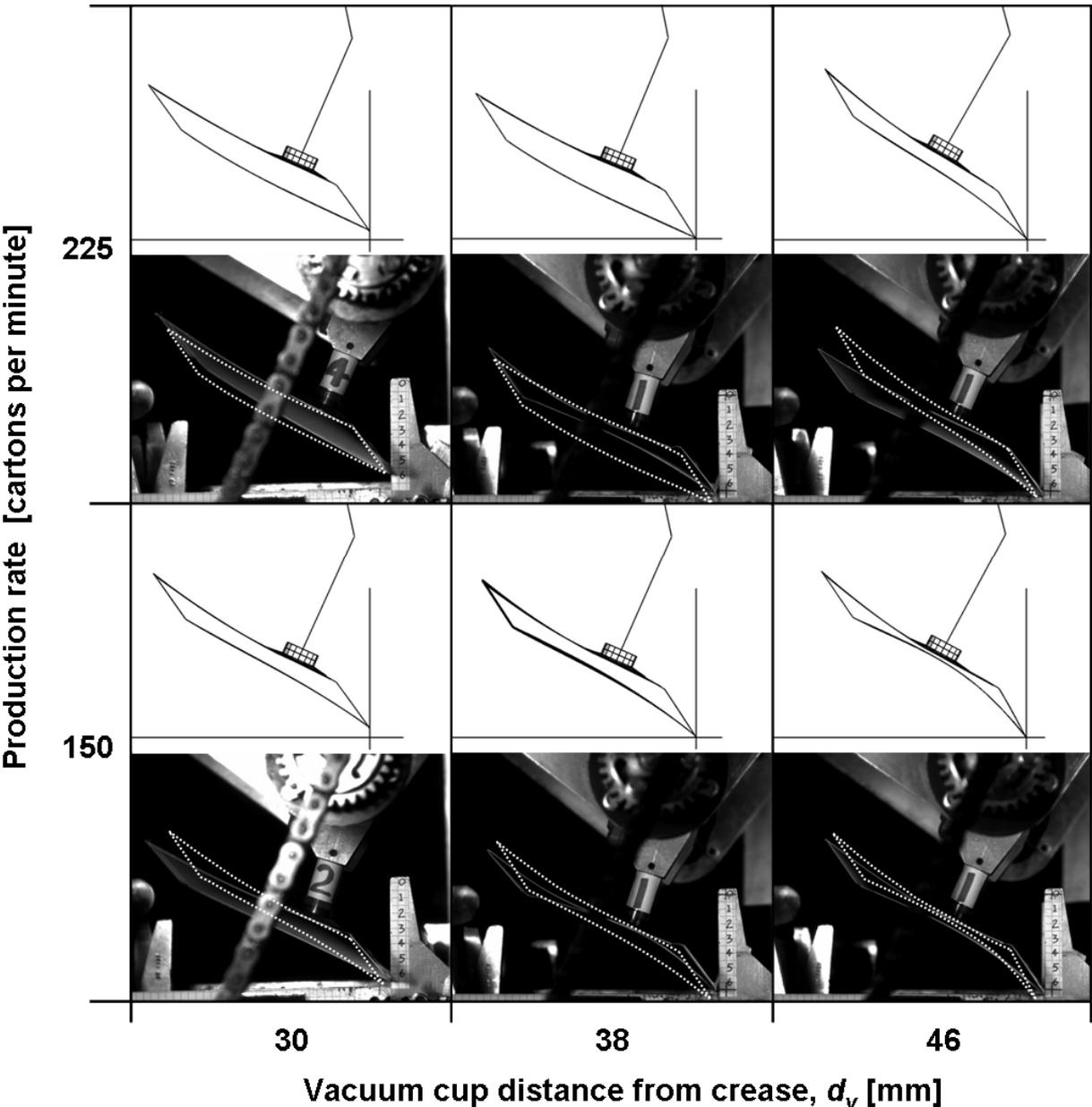
Figure 5. Comparing simulation results with high speed video footage of skillet erection at the three vacuum cup positions considered. Predicted results are shown above corresponding frames from high speed video. Predicted results (dotted line) are superimposed on the high speed video images.
