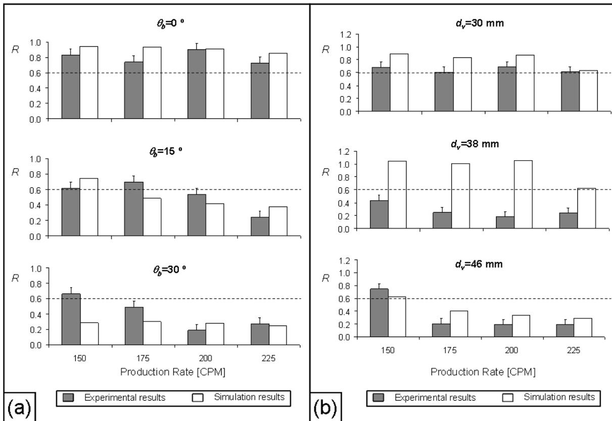
Figure 6. Comparing predicted and experimental values of opening ratio for all backstop angles (a) and vacuum cup positions (b) at all production rates considered.  $R$  values below 0.6 indicate operating configurations in which buckling is in evidence.
