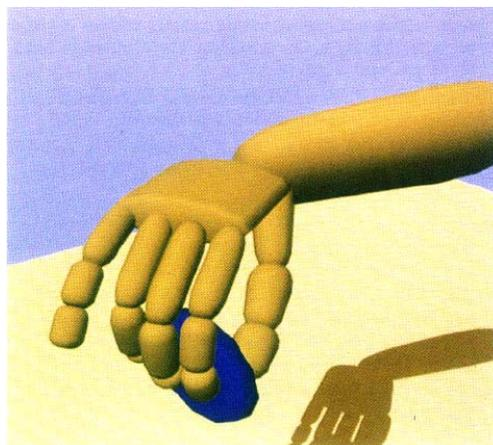
*Figure 3 Grasping simulation with rigid body representation [34].*
