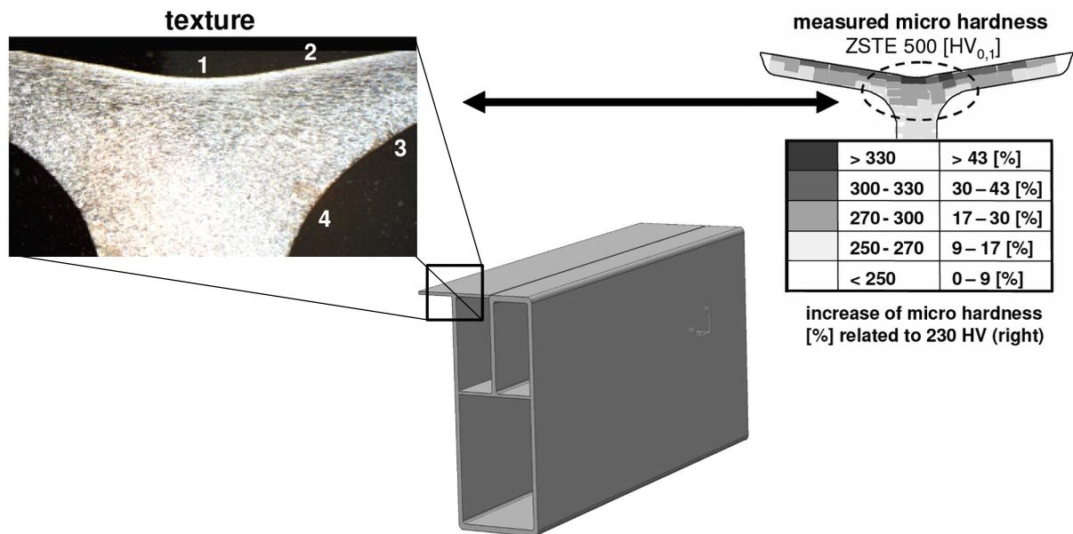
Figure 7: Distribution of the Micro Hardness in the Bifurcated Profile
