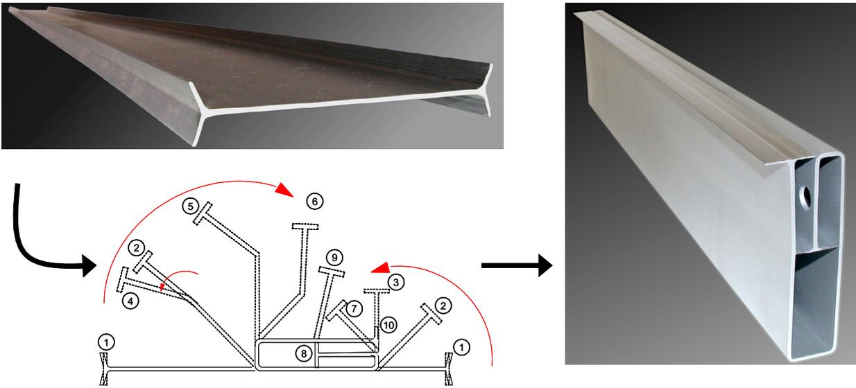
Figure 1. Manufacturing a 3-chambered Profile
