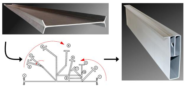
Figure 1. Manufacturing a 3-chambered Profile
