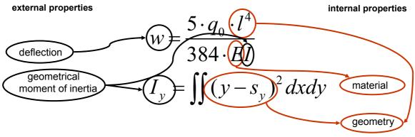
Figure 4. External and Internal Properties
