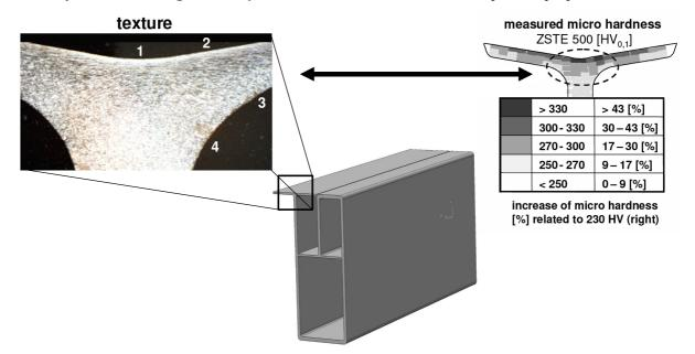
Figure 7: Distribution of the Micro Hardness in the Bifurcated Profile
