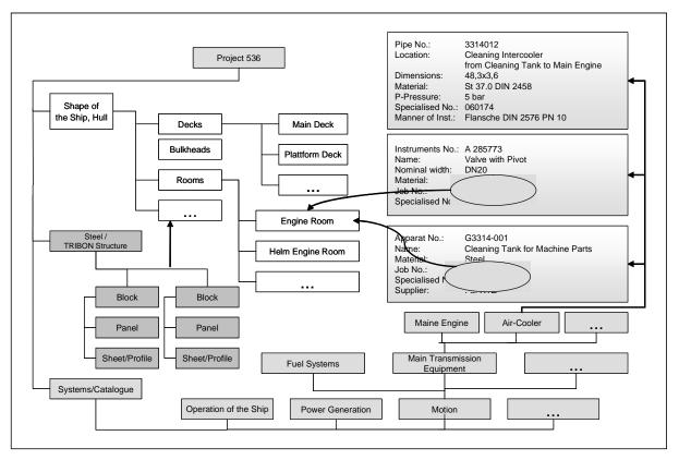
Figure 3. Product data model of a ship
