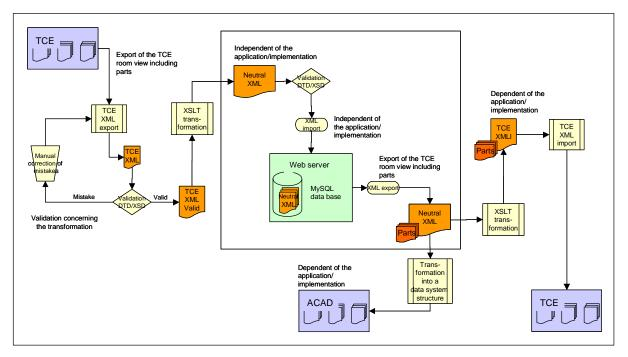
Figure 4. Product data exchange via the internet platform
