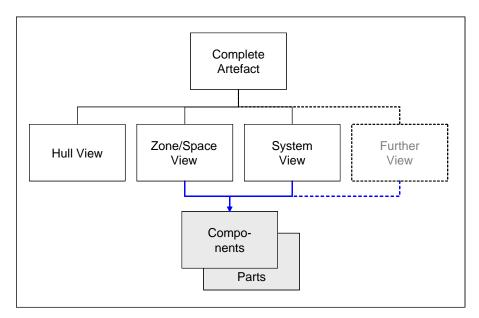
Figure 1. Basic structure of the general product data model
