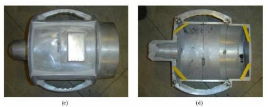
Figure 2: Rheometer-4SCC sample bucket, CAD drawing (a), the final product castedout of aluminium (b), the outside of the mold (c) and the inside of the mold (d)
