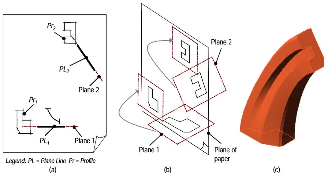
Figure 3. (a) Sketch drawn with PSL (b) projection of profiles (c) 3D model generated
