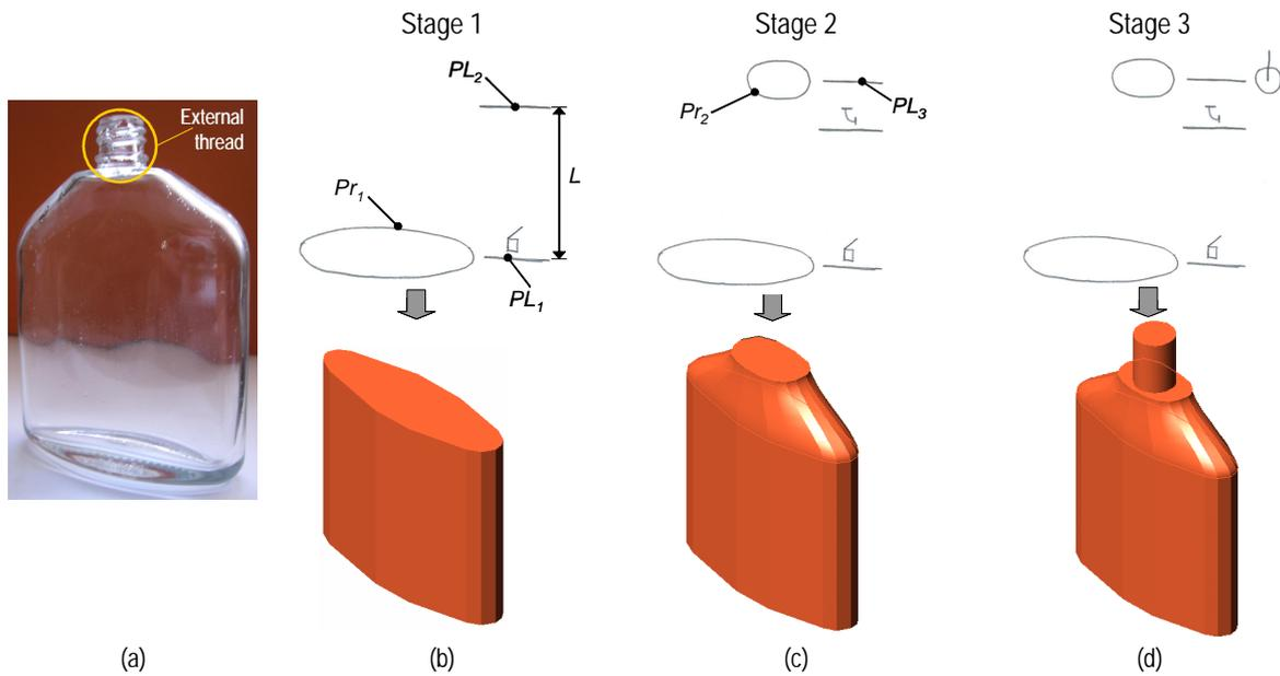
**Figure 5. (a) Physical object (b)-(d) decomposition of its sketch representation & 3D model build-up**
