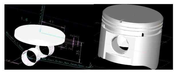
Figure 9. a (left) Example of surface model based design specification model with URL-links to XML-database. b (right) Final product model after foundry related detail design.
