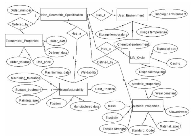
Figure 5. ER-submodel of the non-geometric properties.
