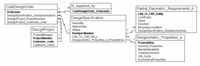
Figure 6. Main level data relation model, created from ER-model in fig. 4.
