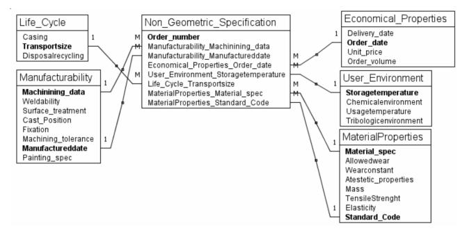
Figure 7. Non-geometric detail level data relation model, created from ER-model in fig. 5.
