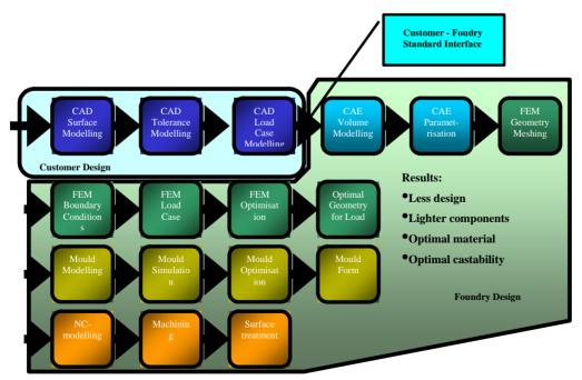
Figure 1. Design process of cast parts
