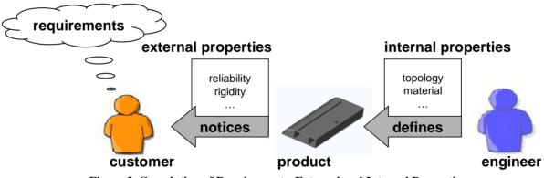
Figure 3. Correlation of Requirements, External and Internal Properties
