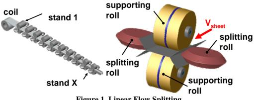
The bifurcations originate from a surface enlargement of the sheet metal's band edge during material forming. Induced high hydrostatic compressive stresses in the local forming zone during the process lead to an increased formability of the material and thereby to the realization of large strains. The bifurcated profile is marked by a bar and two flanges. The surface beneath the splitting roll is defined as the upper side.
