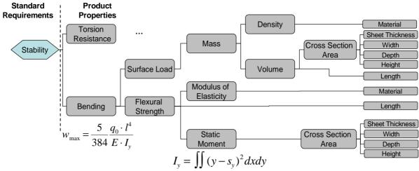
Figure 7. Property-Network of a Cable Conduit
