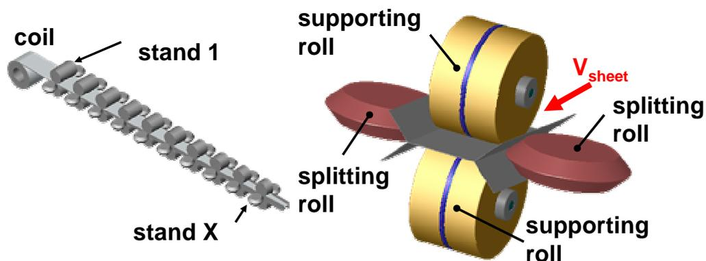
Figure 1. Linear Flow Splitting
