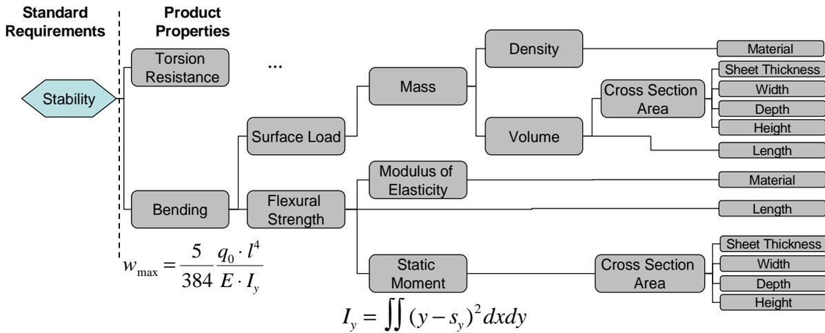
Figure 7. Property-Network of a Cable Conduit
