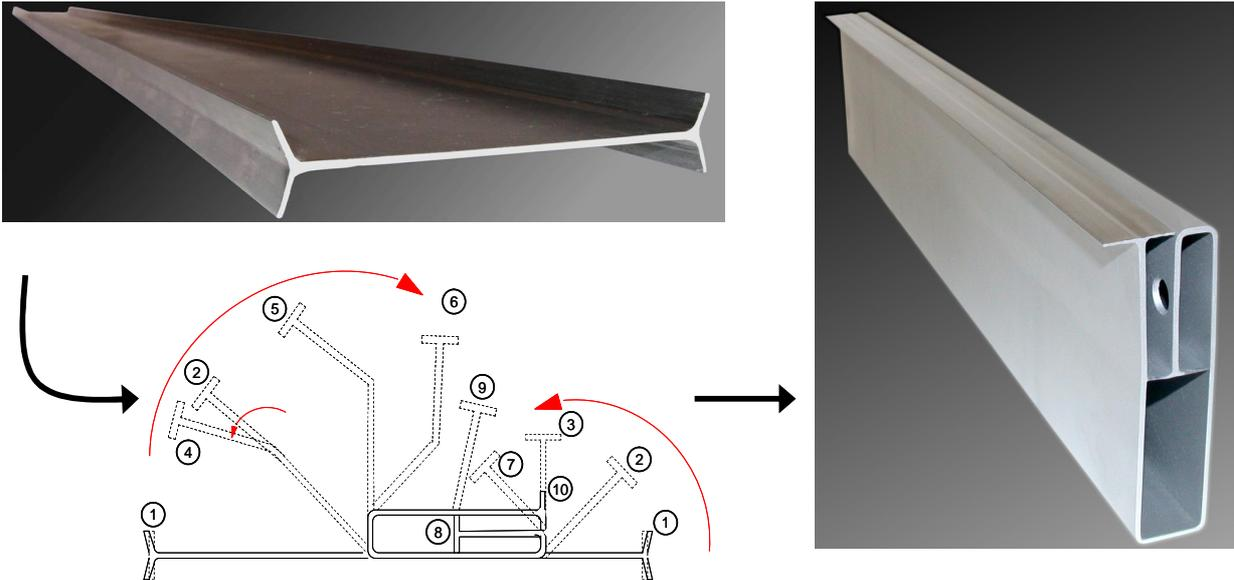
**Figure 2. Manufacturing of a 3-Chambered Profile Structure**
