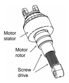
Picture 3. Linear actuator in a prosthetic foot with bionic technology
