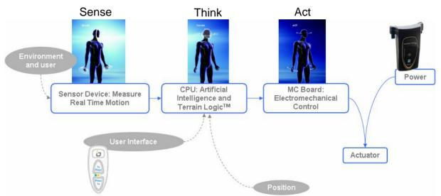
Picture 2. High Level Technical Architecture of a microprocessor controlled prosthetic foot
