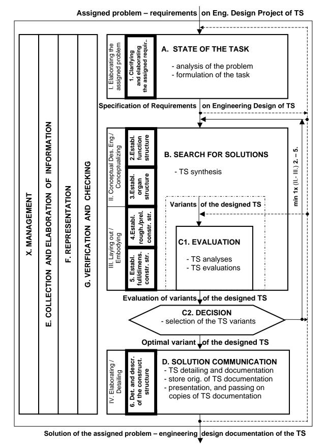
Fig.4: Basic structure of the General Procedural Model of System Design Engineering of TS 1-6 [Hubka 1996 => Hosnedl 2006]
