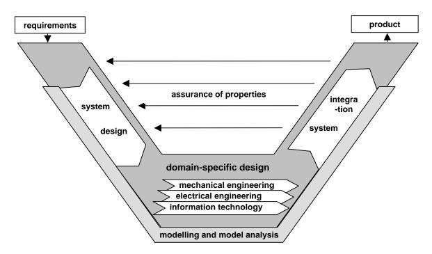
Fig. 1: General V model as a macro-cycle of the generic procedure for designing mechatronic systems [VDI 2004]
