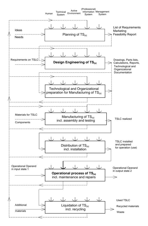
Fig. 2: General model of Life Cycle (LC) of Technical Product / System (TS<sub>(s)</sub>) as a cycle of Transformation Processes (TrfP) and corresponding Transformation Systems (TrfS) [Hubka 1988]
