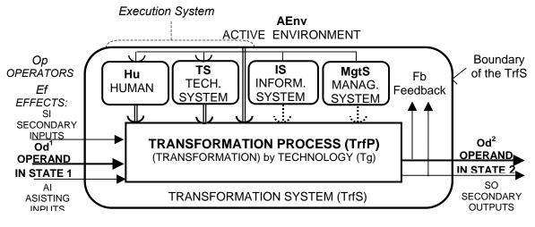
Fig. 3: General Model of the Transformation System (TrfS) with Transformation Process (TrfP) [Hubka 1988, etc.]
