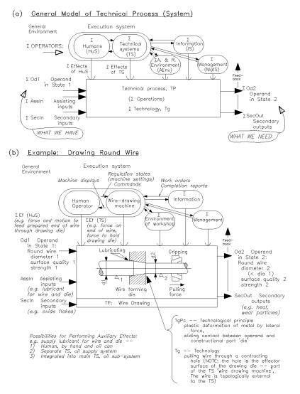
Figure 4. Example: Wire Drawing
