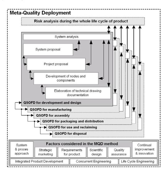
Figure 4. Meta-Quality Deployment method [Blecha 2004]
