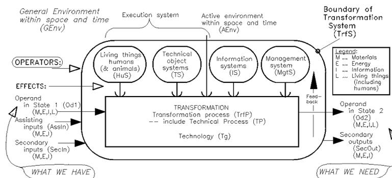
Figure 1 General Model of a Transformation System
