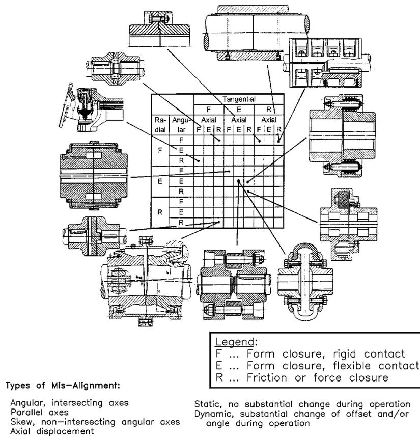
Figure 12 Classification of Couplings according to Closure Principle
