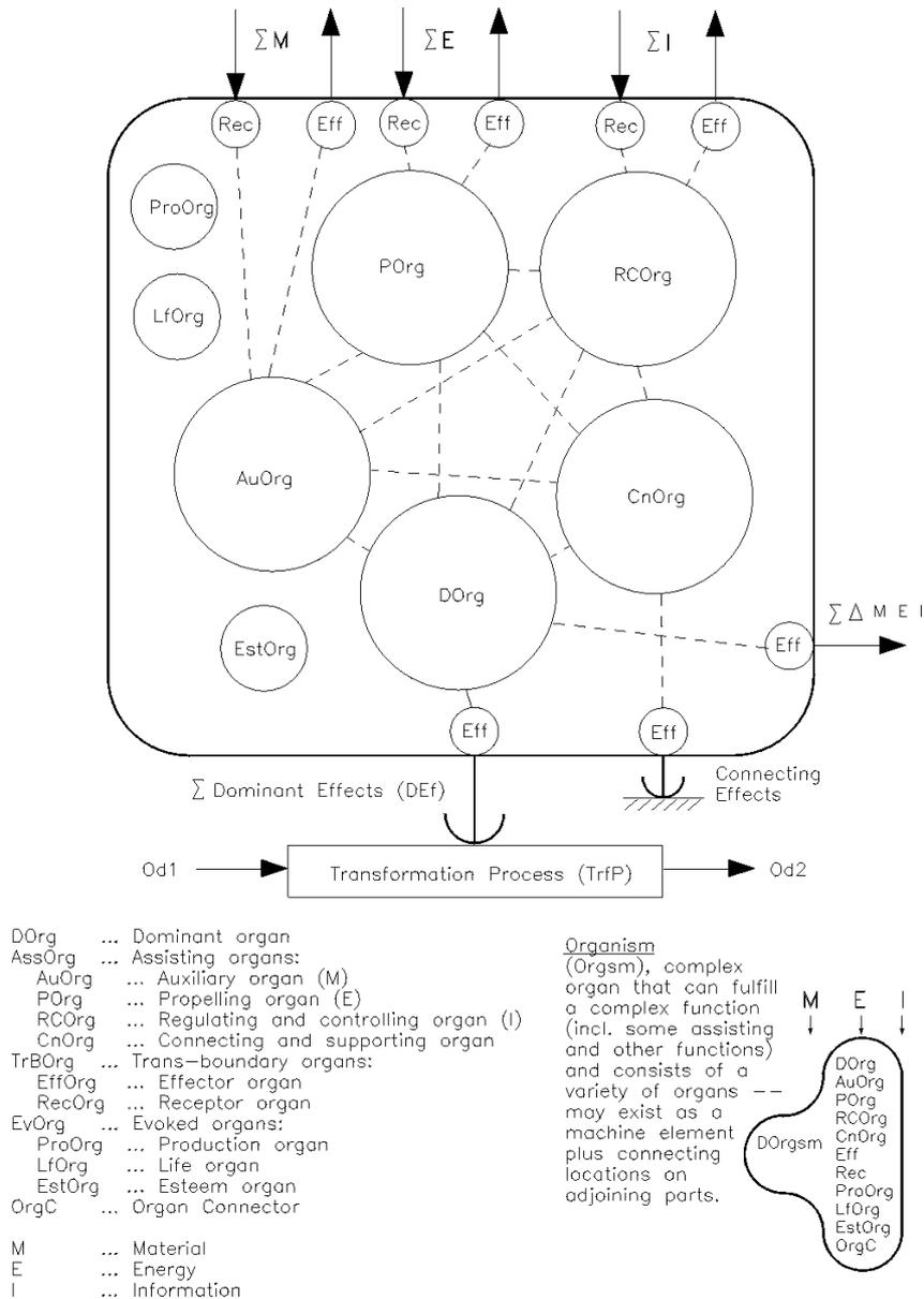
Figure 5 Model of the Organ Structure of Technical Systems
