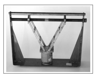
Figure 3. A student engineer's can crusher
