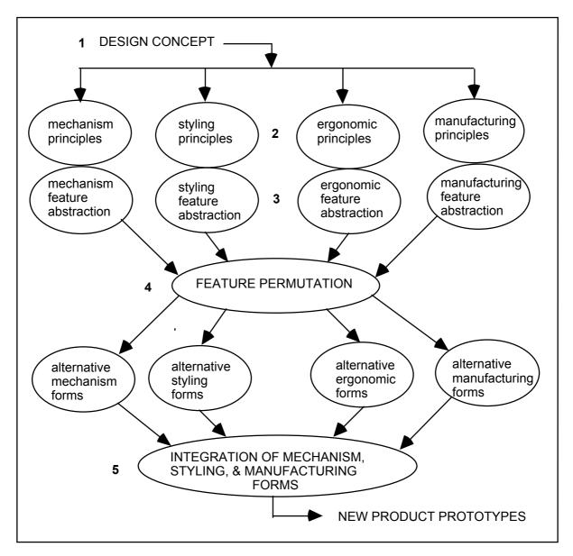
Figure 6. A structured design process
