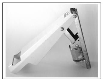
Figure 2. A proprietary can crusher
