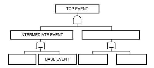
Figure 5. FTA scheme/diagram
