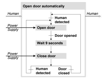
Figure 5. Second function structure of an automatic door opener.
