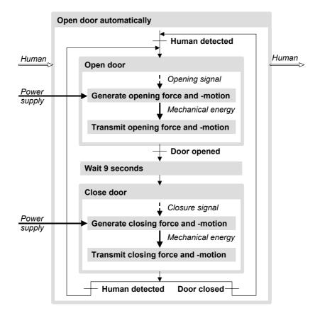
Figure 6. Third function structure of an automatic door opener.
