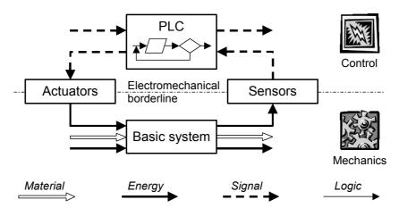
Figure 2. Schematic layout of a mechatronic system controlled by a PLC.
