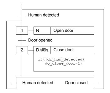
Figure 7. SFC derived from the third function structure.
