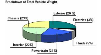
Figure 1. Breakdown of Total Vehicle Weight [2]
